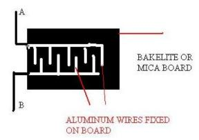
If there is no rain, the resistance between the wires will be very high and there will be no conduction between the wires in the sensor. If there is rain, the water drops will fall on the rain sensor which will also decrease the resistance between the wires and wires on the sensor board will conduct and trigger the NE555 timer through the transistors circuitry. Once NE555 is triggered, it will make the output pin high and which will make the buzzer to make alarm.
